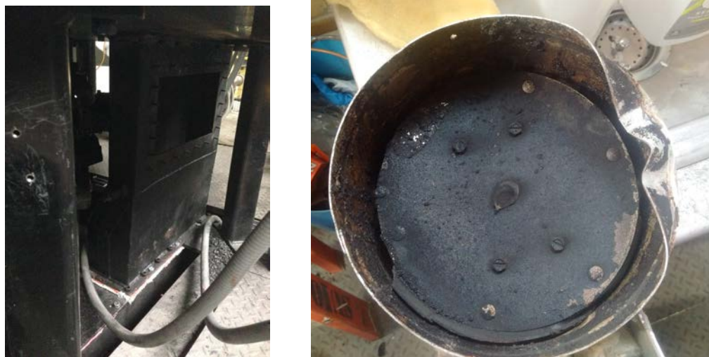
Figure 2.11: Previous chute (left) and damper (right) damper installed in the UI gasifier
